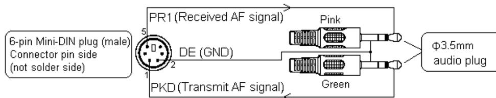
Serial communications cable (for PC RS-232C serial port) pin configuration
